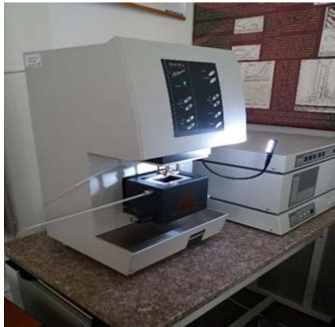
Fig. 2. DMA analyzer used for experiments
