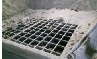
Fig. 10. Rolling collector equipped with grill, mesh size 0.40 X 0.40 m
