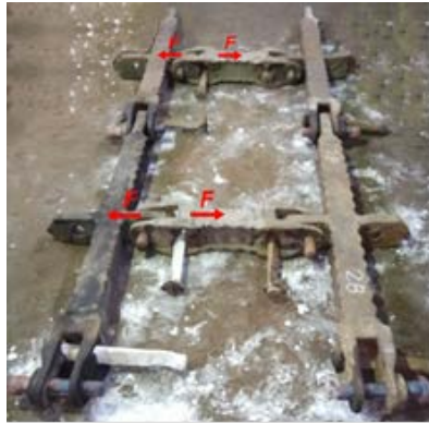
Fig. 3. Coupling between the beams GSA-1250S and the spacers GSA-570S [15]
