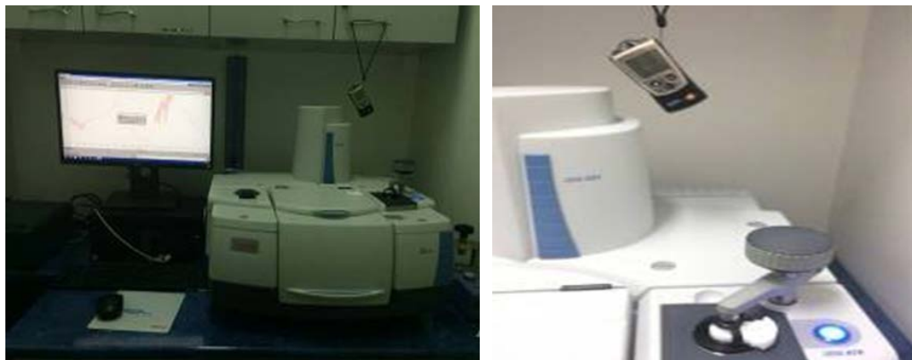
Fig. 1. (a) Nicolet IS50 Infrared Spectrometer equipment; (b) ATR module with diamond crystal and device for analyze of volatile substances.
